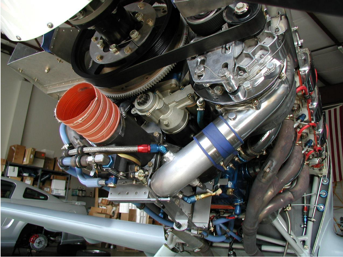
Installation on a super charged 540. The fuel control is installed on the inlet side of the super charger compressor.
