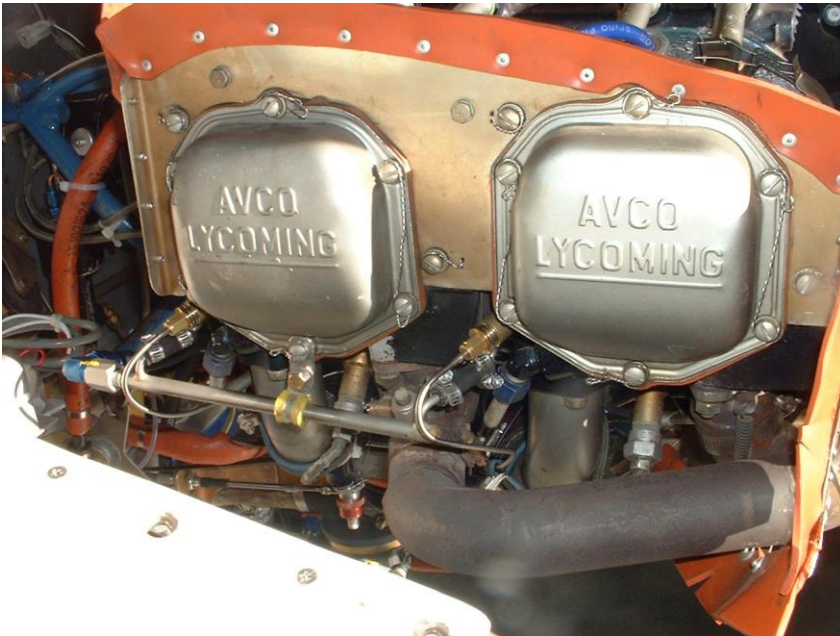
Long EZ Bleed Air Rail installation.
