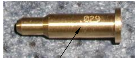
Restrictor marked with size
