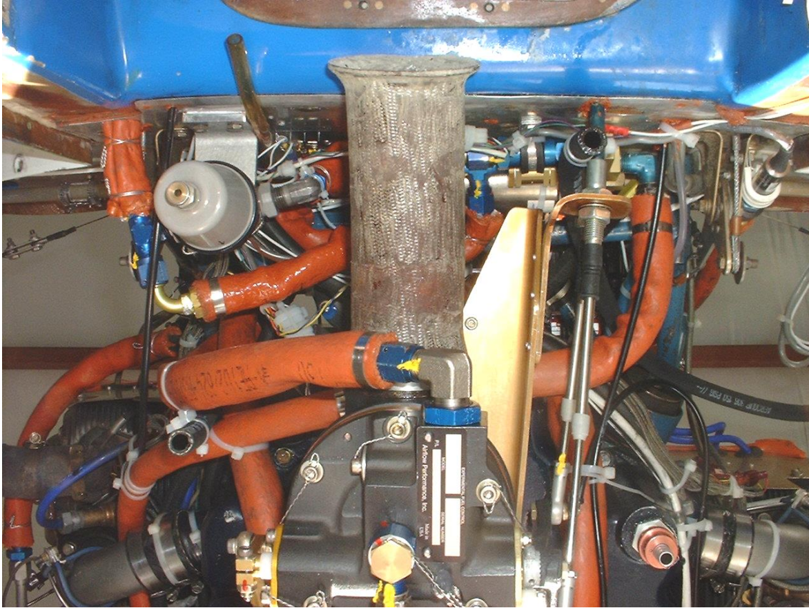
Composite air inlet attached to FM-100 in Long EZ installation. Air inlet points into duct that feeds cold air into the engine compartment.
