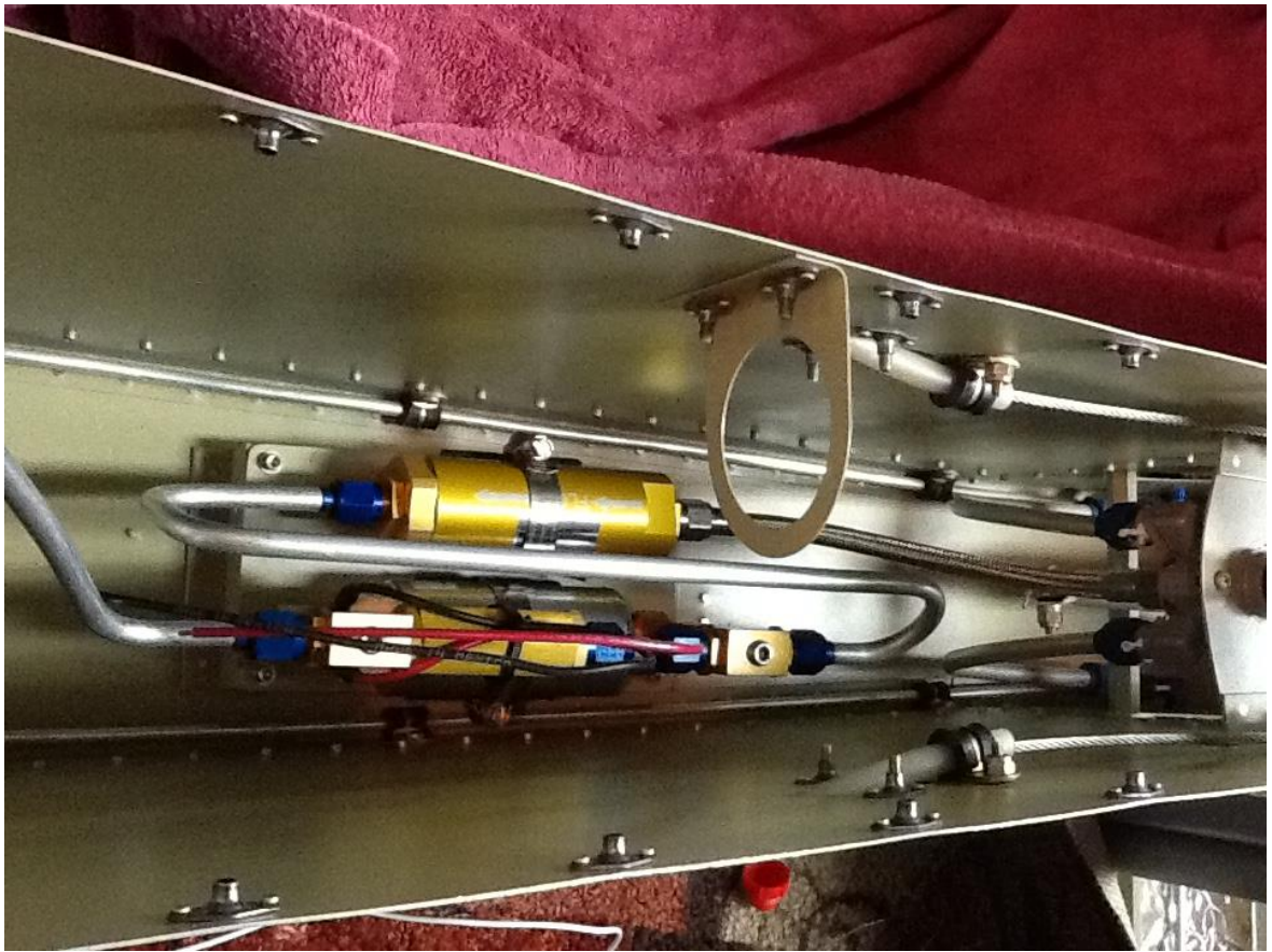
Boost Pump and Filter mounted in the tunnel of an RV-10
