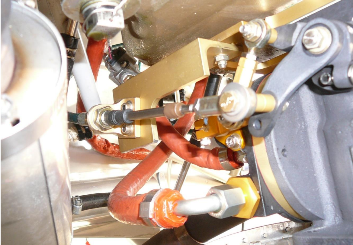
Throttle and Mixture Control cable hook-up on RV-8 360 up draft sump.
