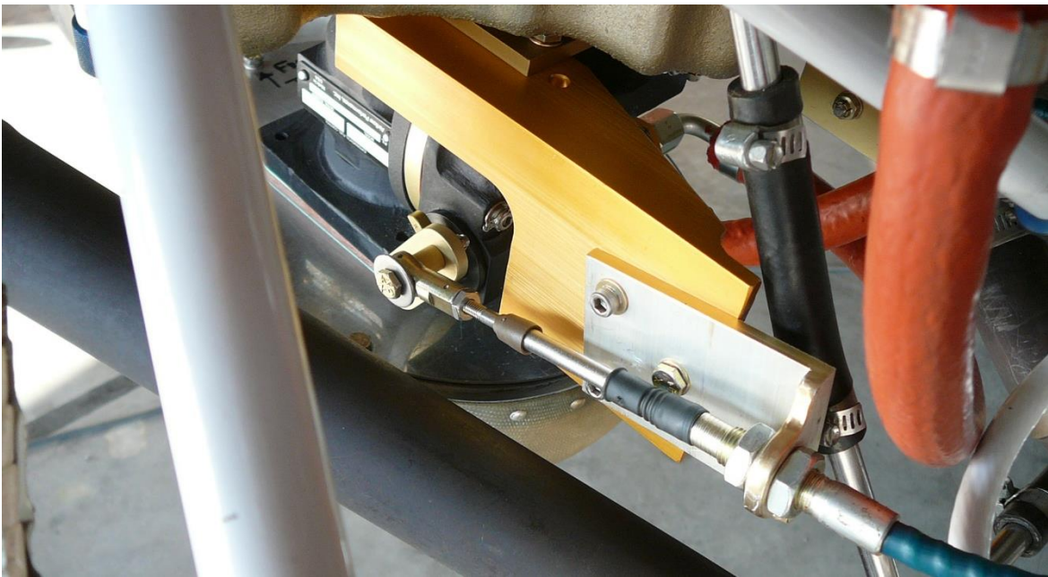
Throttle and Mixture Control cable hook-up on RV-8 360 up draft sump.
