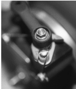
Mixture control in ICO position
