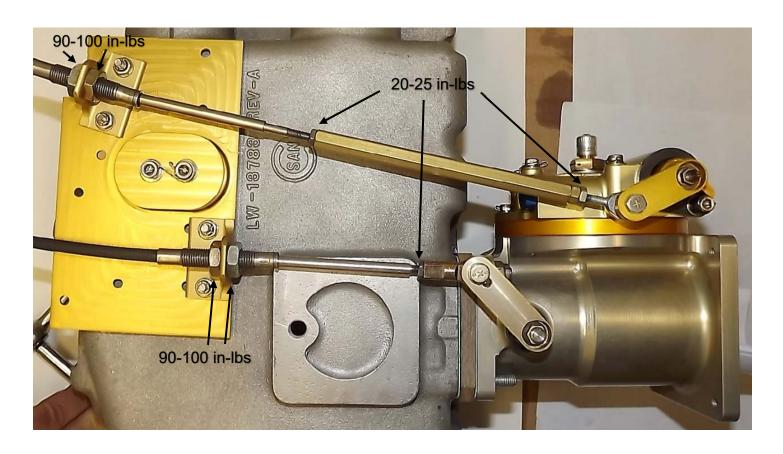
After cable rigging is verified, torque 11/16" cable jam nuts to 90-100 in-lbs. Torque 10-32 rod end jam nuts to 20-25 in-lbs.
