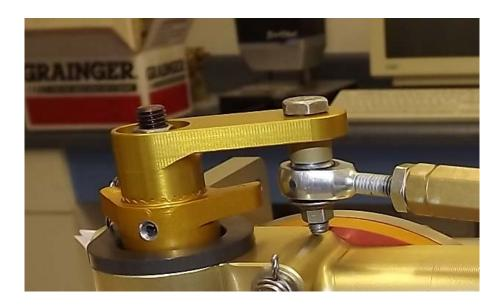
Ensure cable rigging is correct to allow complete travel from Full Rich to ICO (Idle Cut Off).
