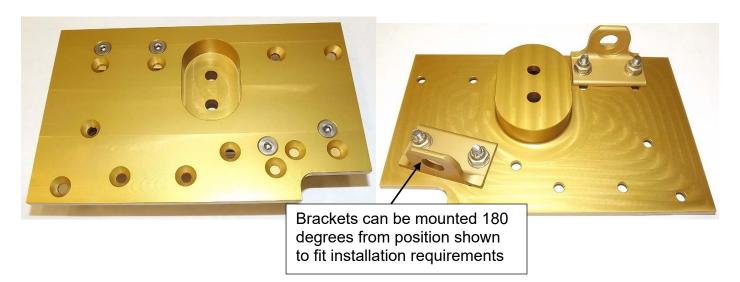
Install the 390 Throttle Mixture Bracket, P/N 3090120 on sump as shown. Secure the bracket with the two  $\frac{1}{4}$ -20 x 3/4" screws, P/N HW-0344-SSD provided. Torque cap screws 35-40 in-lbs. Lock wire the screws in accordance with AC43-13.
