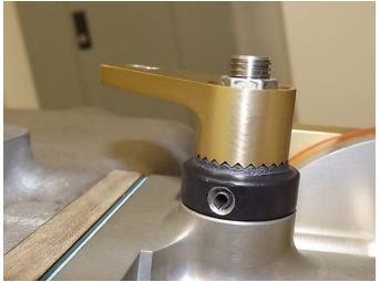
Attach the Throttle Cable to the cable bracket as shown. Use the jam nuts to secure the cable in place. **Depending on rigging, your installation may differ slightly from the picture below.**
