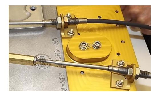
Install the jam nut and rod end bearing on the cable. Connect the rod end and cable to the throttle lever using the AN3-7A bolt provided with the kit and 1 standard thickness washer, P/N AN960-10 either side of the lever. Install the thin large area washer next to the lock nut. Secure the bolt in place using the MS21042-3 lock nut. Torque lock nut to 25-30 in-lbs.
