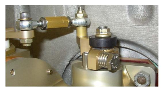
Remove existing studs from the sump and install the provided 5/16-2 Studs ST-18, P/N HW-1904. Spray studs with Loctite Primer SF 7471 and allow to dry. Apply Loctite 620 to threads prior to installing the studs. The studs should extend approximately 1.19"-1.4" from the front of the sump when properly installed.
