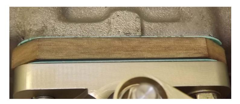
With the studs, gaskets and phenolic spacer installed, mount the FM-150 Fuel Control to the sump as shown. Secure the fuel control to the sump using AN960-516L washers and 5/16 Locknuts, P/N MS21045-5 provided. Torque 5/16 lock nuts to 110-115 in-lbs.
