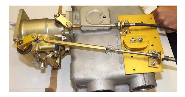
Position mixture control lever to ensure correct rigging and operation. Attach the rod end to the mixture lever using the AN3-10A bolt provided (there is no washer between the head of the bolt and the lever). Install the .19" spacer between the rod end and lever. Install the thin large area washer between the rod end and lock nut and secure. Torque lock nut to 25-30 in-lbs.
