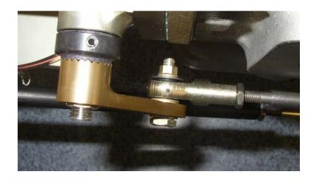
Adjust cable to insure full travel of the throttle. At the WOT position the throttle does not have to hit the stop hard. 1/16" clearance is preferred so that the throttle stop lever does not get worn out.
