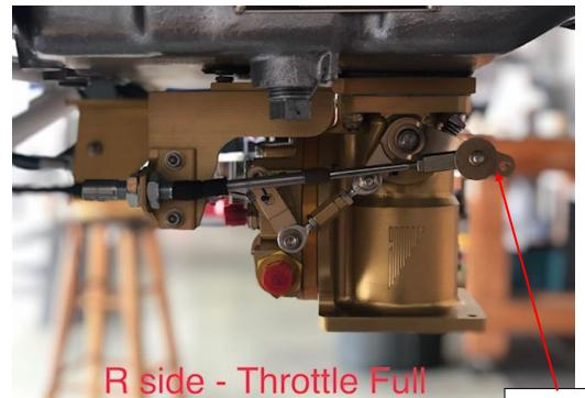
Use the appropriate hole to achieve full travel for the type of quadrant or push pull cable used.
