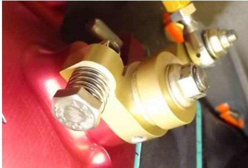
Throttle Stop Lever shown at idle position
